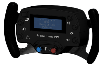
(b) Custom CFRP and 3D-printed steering wheel with integrated regenerative braking paddle.
