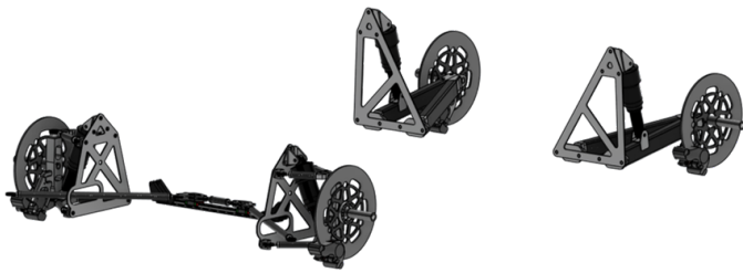
(a) Full suspension and steering assembly: double-wishbone front corners, trailing-arm rear, and the central steering linkage.
