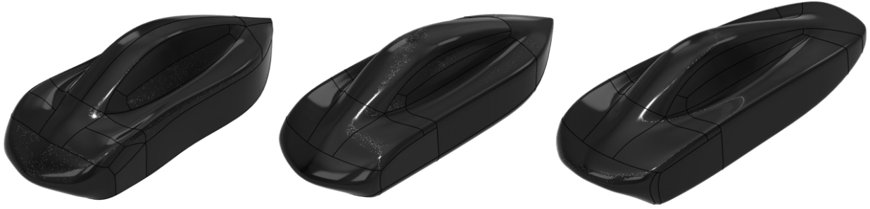
(a) Body geometry at iterations V1, V3, and V7, showing progressive refinement toward the final minimal fastback form.
